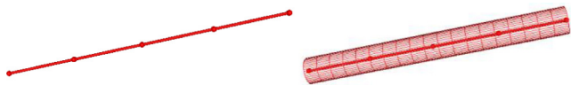
Fig. 3. Yarn (10 mm) having 5 nodes, yarn centre line (left), yarn render model (right).
