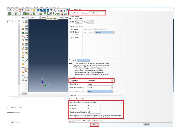
Definition of the viscoelastic homogenization step
