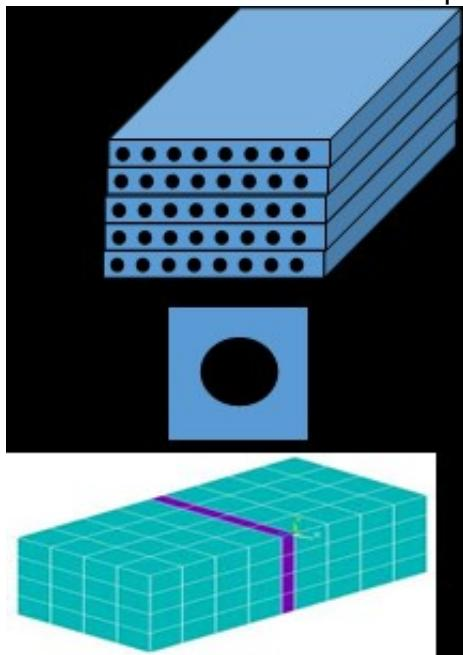
Let the material properties of the fiber and matrix be: Fiber:  $E_{11} = 230 \text{ GPa}$ ,  $E_{22} = 15 \text{ GPa}$ ,  $G_{12}=G_{13} = 15 \text{ GPa}$ ,  $G_{23} = 7 \text{ GPa}$ ,  $\nu_{12}=\nu_{13} = 0.2000$ ,  $\nu_{23} = 0.0714$ .
