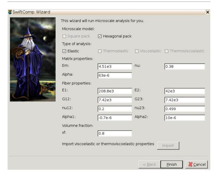
Note the CTEs will not be used for the elastic analysis. Click finish and the microscale homogenization will be performed and the results will be automatically pop up
